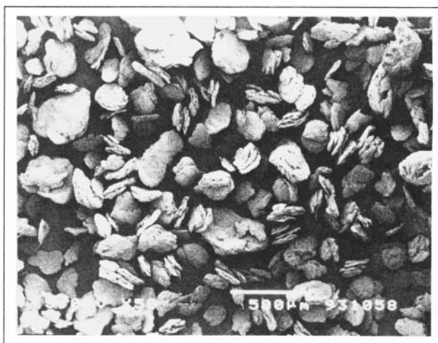
Figure 7. SEM photograph of phenanthrene with 5 h growth time, without a pressure pulse and 900 rpm, exp. no. 86.
